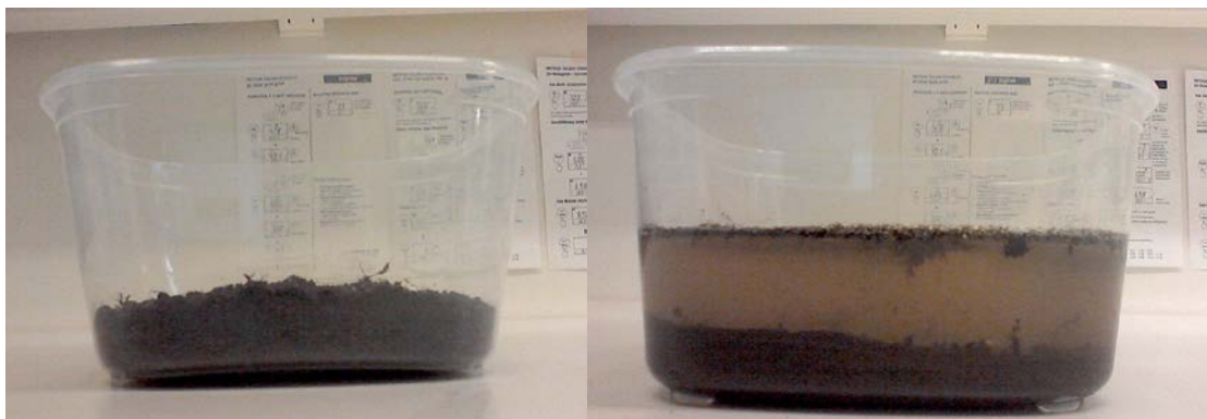
Figure 7. Left: a plastic container filled with approximately 2 cm of soil. Left: a plastic container tiller with the double amount of water, (Adriaan van Tour, 2015).
