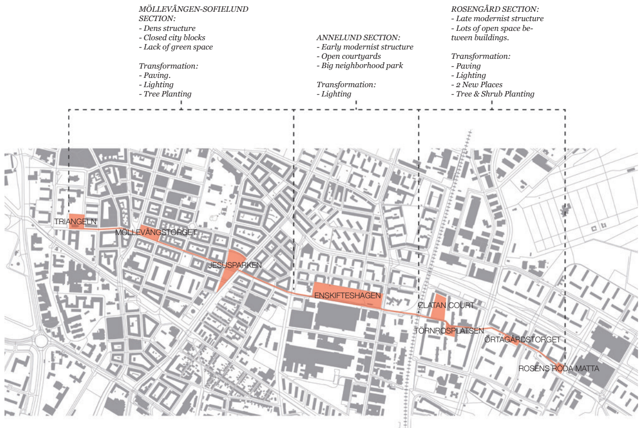
Fig 16. Rosengårdsstråket and its 3 sections. Three specific sections and the main transformation work made.
