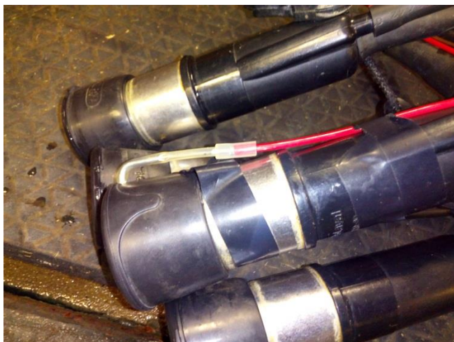
Figure 8. Measuring point mouthpiece chamber. Stainless steel pipe inserted through the liner wall.
