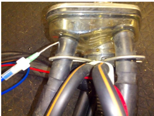
Figure 7. Measuring point claw bowl chamber. Hypodermic 14-gauge needle introduced through the short milk tube, leading inside the claw bowl.
