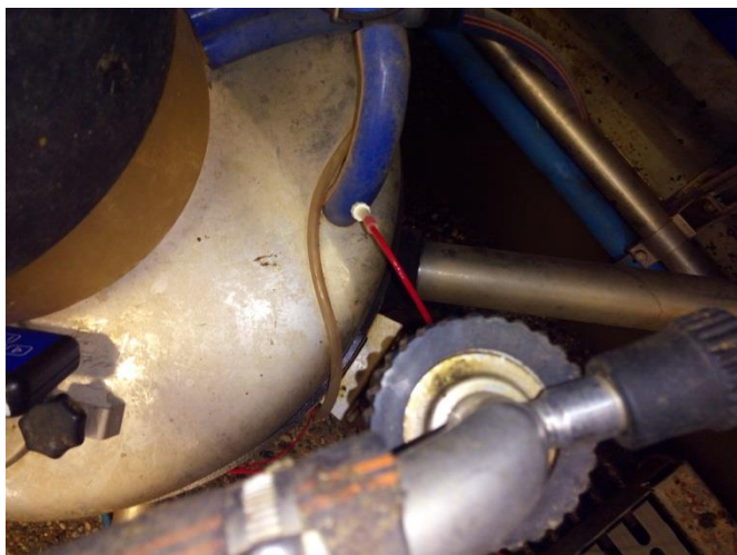
Figure 5. Measuring point receiver. Vacuum meter connected to the measuring point by a 2m tube and a 14-gauge hypodermic needle.
