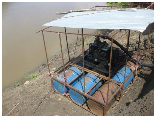
Figure 10. A good example of a solution to a problem – the floating pump station in Kakora. (Photo: Agnar Kjeller).
