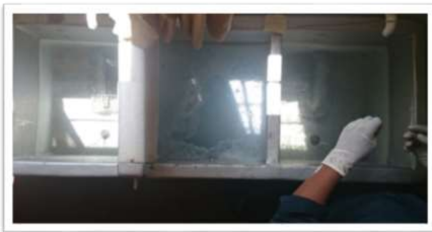
Figure 4. Fibres are washed in three steps. Photo: Jakob Killander
