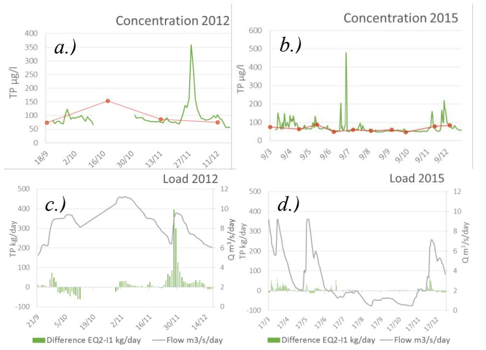
Figure 20. Plots showing a comparison between two load estimation methods (EQ2 and I1) 2012 and 2015. Graph a and b describe concentration TP over the period when the sensor was in the water, red line and dots symbolize grab samples and linear interpolation while the green line represent high frequency TP. The graphs c and d are describing the difference between the load from EQ2 and I1 on the left y-axis (green staples), the right y-axis (grey line) is describing flow.
