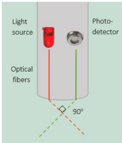
Figure 7. Components of the sensor showing angle from the near infrared light source and the light observed by the photodetector. Information from YSI, 2016.
