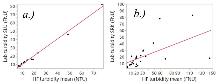
Figure 14. Plots showing linear regression analyses with turbidity from grab samples and HF turbidity mean (1h). Graph a: grab samples analysed in the lab taken at the time of managing the sensor (SLU), graph b: grab samples (SRK) compared to HF turbidity.
