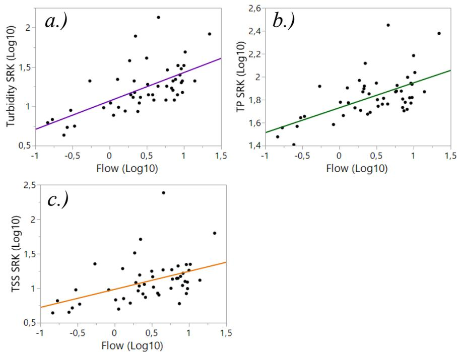
Figure 13. *Plots of flow vs turbidity (a), TP (b) and TSS (c). Data from grab sampling (SRK).*
