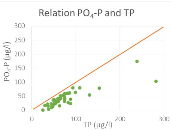
Figure 11. Relationship between  $\text{PO}_4\text{-P}$  and TP (green markers), red line represents the 1:1 ratio.
