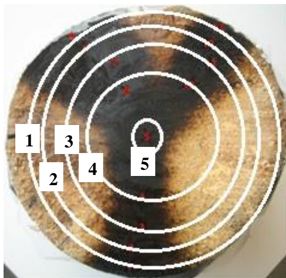
Figure 2 Sampling locations on the sections. Where the outermost samples being in ring 1, second outermost in ring 2, third outermost in ring 3, fourth outermost in ring 4 and ring 5 being the centermost samples.
