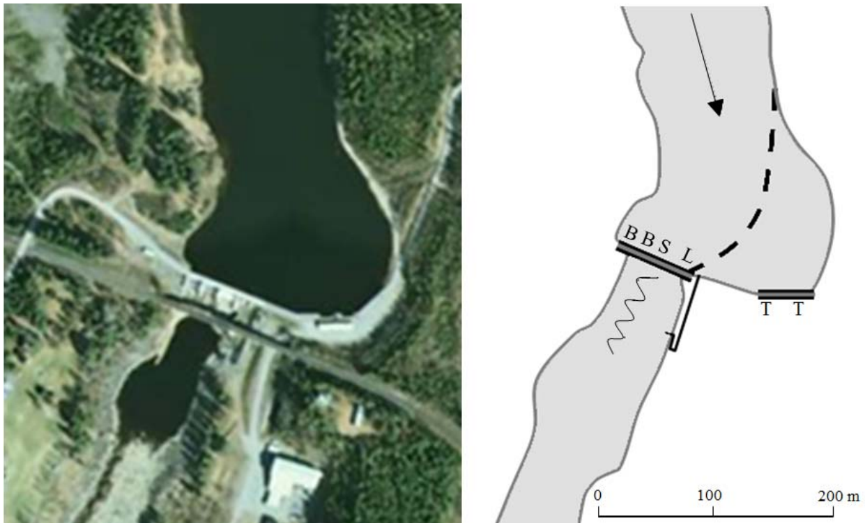
Figure 2. An up close picture of the power station with the different openings marked (B=bottom spill, S=surface spill and L=fish ladder and T=turbine intake), the dashed line shows the placement of the guidance structure and the arrow shows the direction of the river flow.
