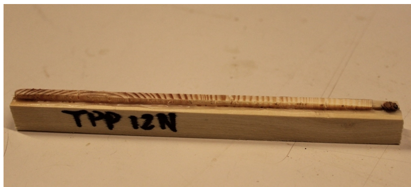
Fig. 10. Pine core mounted on wooden stick and sanded
