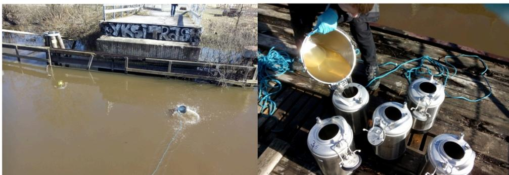
**Figure 7:** Sampling of river water downstream and transfer of sampling water into stainless steel containers.
