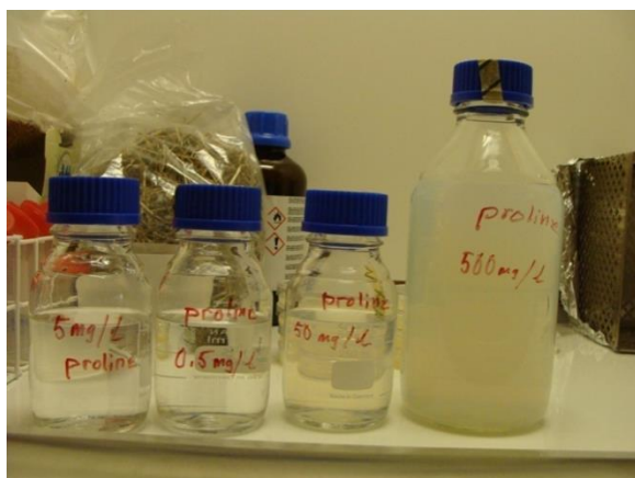
Photo 13: Tenfold dilution series of Proline®. Field dose (500 mg/l), dilution 1/10 (50mg/l), dilution 1/100 (5 mg/l) and dilution 1/1000 (0.5 mg/l)
