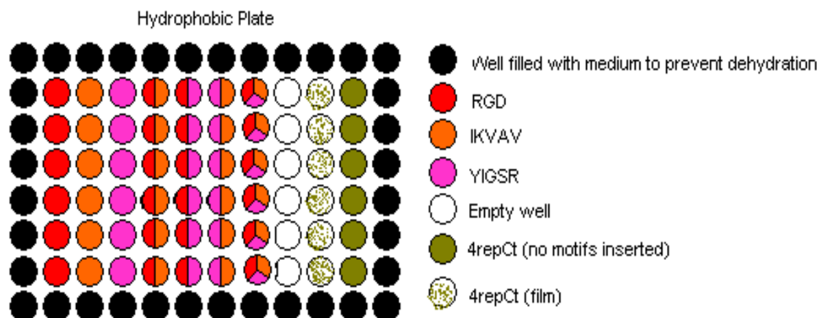
Fig2: There are 10 rows with 6 wells each on the hydrophobic plate. The ten rows are hydrophobic (nothing added), 4repCt (film), 4repCt (foam), RGD4repCt (foam), IKVAV4repCt (foam), YIGSR4repCt (foam), RGD + YIGSR4repCt (foam), IKVAV + YIGSR4repCt (foam), IKVAV + RGD4repCt (foam) and RGD + IKVAV + YIGSR4repCt (foam). Around the rows wells are filled with medium to prevent evaporation of water. On the hydrophilic plate (not pictured), a 3x2 area is surrounded by medium filled wells, and the six wells inside is a negative control using hydrophilic wells.
