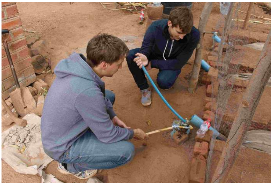
Figure 20: Extraction of sample from digester outlet to be brought back to the lab for further analysis.
