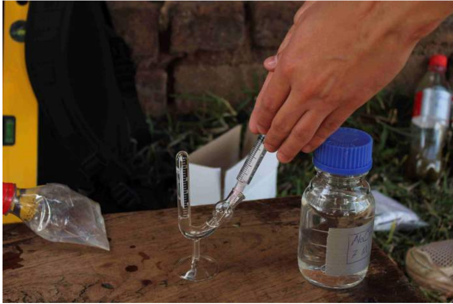
Figure 17: The gas was injected from the syringe into a Dr. Einhorn's Fermentation Saccharometer.
