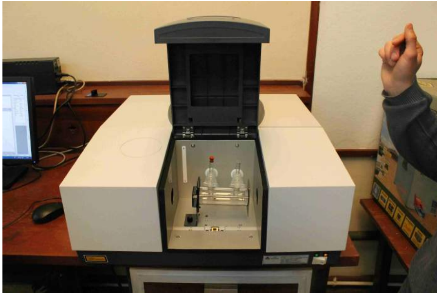
Figure 19: Gas sample in the spectrophotometer ready for analysis.
