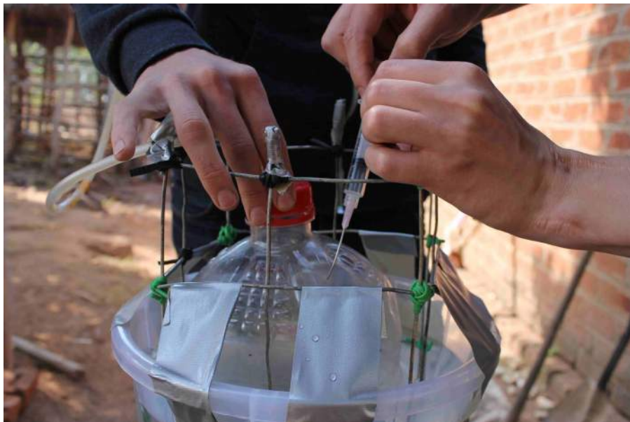
Figure 16: The gas sample was collected from the gas volume measuring device using a small hole in the upside down container.
