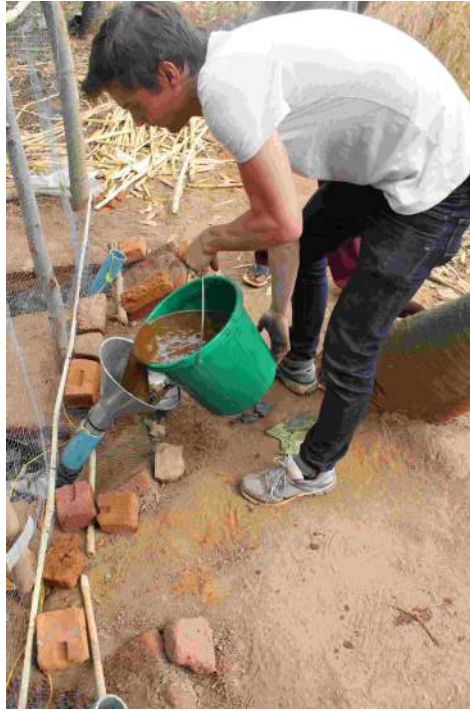
Figure 13: A funnel was made in order to simplify the process of filling the digesters. The slurry is a mix of cow and goat manure with added water .
