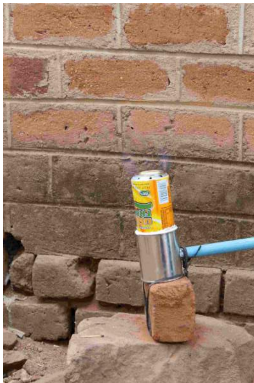
Figure 22: The first prototype of the burner with which we were able to test that a burnable gas was being produced in the digestion process.
