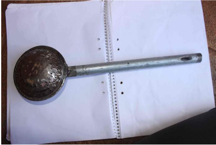
Figure 23: The later designed biogas burner with air and gas intake.
