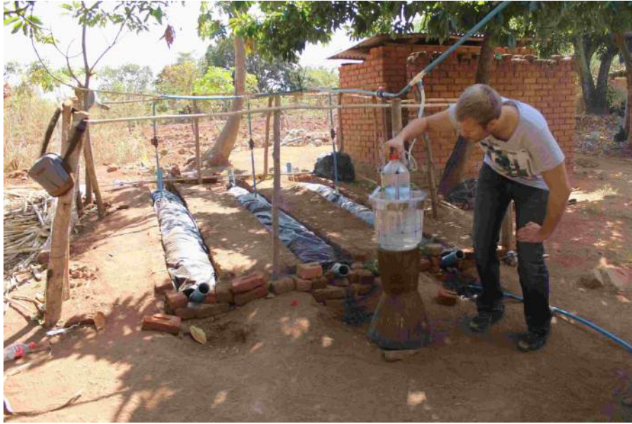
Figure 15: The upside down container was manually raised in the larger bucket and thereby creating a suction that pulled the biogas from the digesters to the gas volume measuring device.
