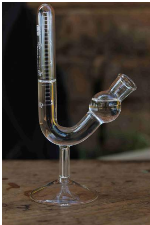
Figure 18: On this picture it is clearly visible how much methane is in the biogas since the methane forms a bubble at the top of the Dr. Einhorn's Fermentation Saccharometer and the carbon dioxide is dissolved in the solution.
