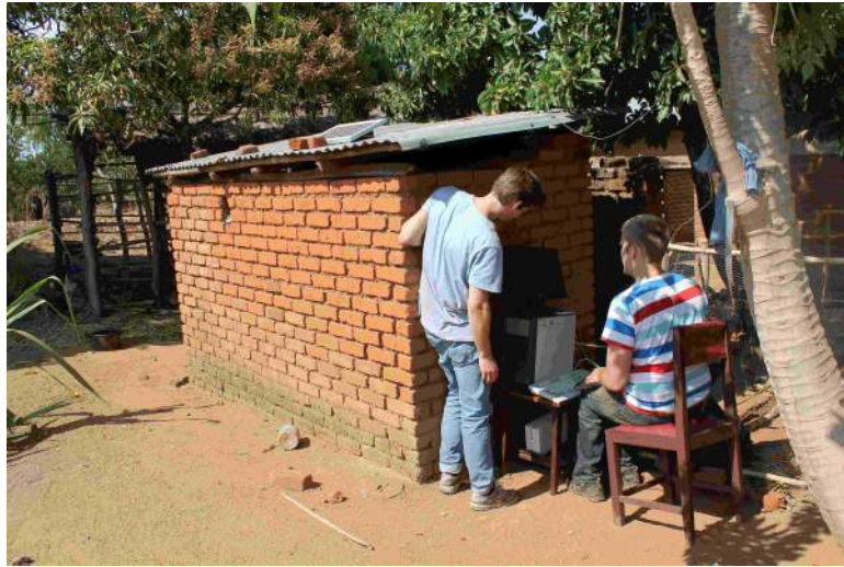
Figure 21: A computer and an external battery was brought to the site in order to collect the data from the data logger. On this picture one can also see the solar panel on the roof used to power the data logger.
