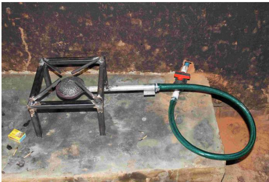
Figure 24: The complete stove with support frame. The biogas enters from a pipe connected to the main system outside the kitchen wall.
