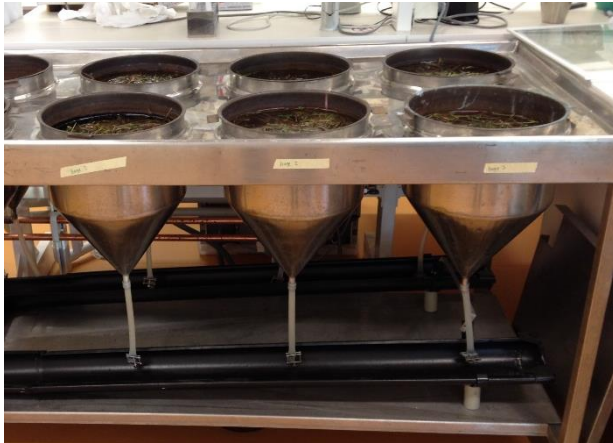
Figure 3. Large Baermann funnels for collection of larvae in grass. Photo by Johanna Karlsson.
