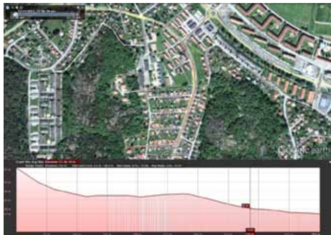
Figure 90. Profile and plan view of the path between a major natural stream and where it could connect to a daylighted stream along Björlandavägen as described in the Location 1 proposal
