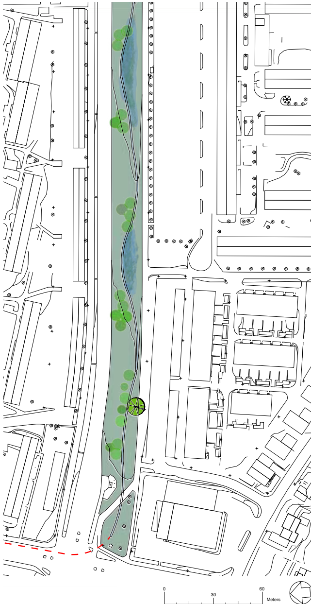
Figure 78. Existing ground profile of corridor: Stormwater from half the road drains onto the wide grassy area. The other half of the crowned road goes in to the combined sewer system.
