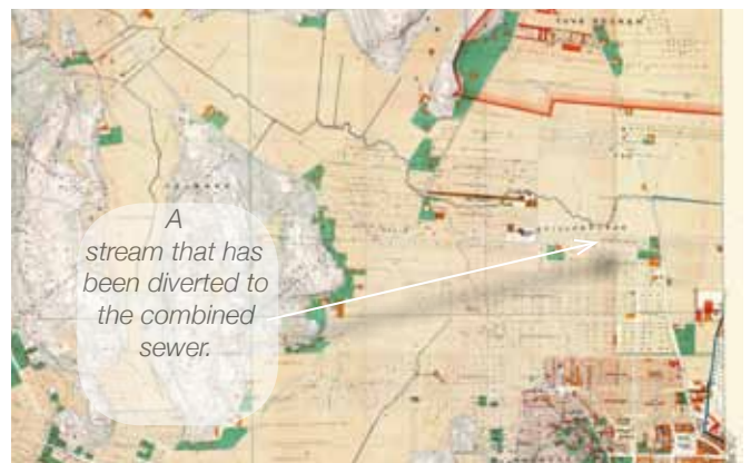
Figure 52. Here you can see a natural stream also called Kvillebäcken here, even though it is actually a tributary to Kvillebäcken coming down from another valley. This water now drains into the combined sewer and is pumped to the sewage plant rather than draining into Kvillebäcken. Today this area has problems with sewage backing up into peoples basements.
