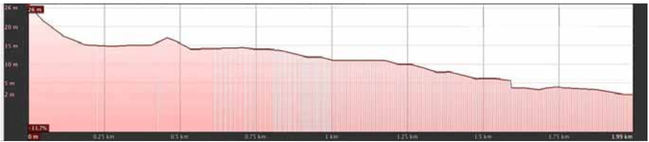
Figure 76. Existing ground profile of the proposed stream. The stream would descend 24 meters over the two kilometer distance from Hising's Park to Kvillebäcken..
