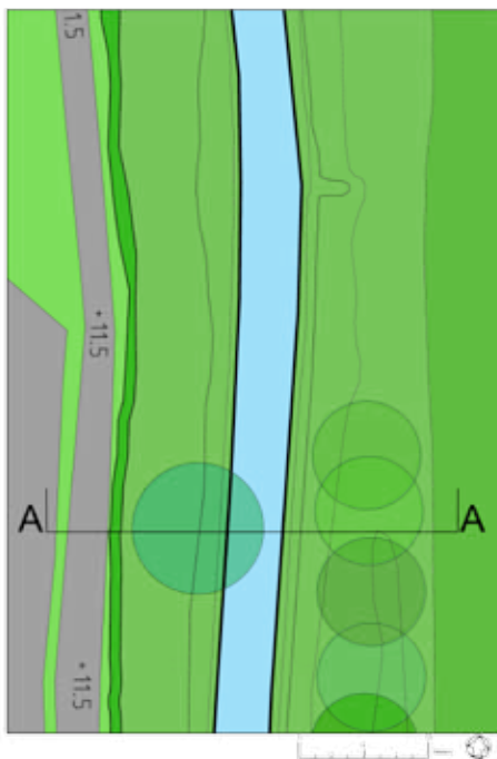
Figure 87. The plan view of a part of the proposed design area. The lower lip of the level spreader follows a contour line so that when water goes over the edge it will run into the riparian edge as sheet flow.
