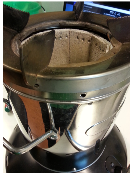
Fig. 9. Removing upper case of stove.
