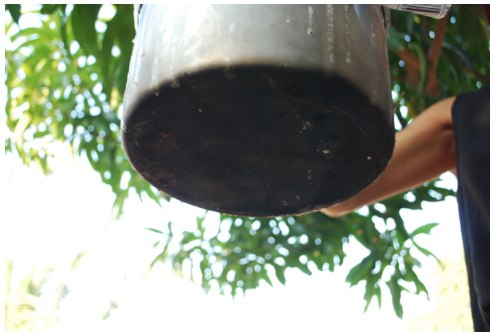
Fig. 22. Unoptimized stove results in black pots after use with wood pellets.
