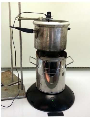
Fig. 12. Setup in fume hood with digital thermometer attached to a stand.
