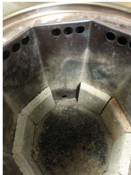
Fig. 11. Rotating lower tiles of stove.
