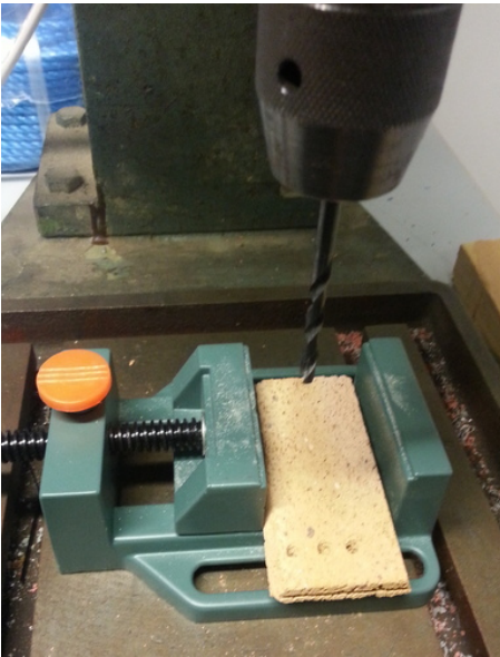
Fig. 8. Enlarging size of air holes in upper tiles.
