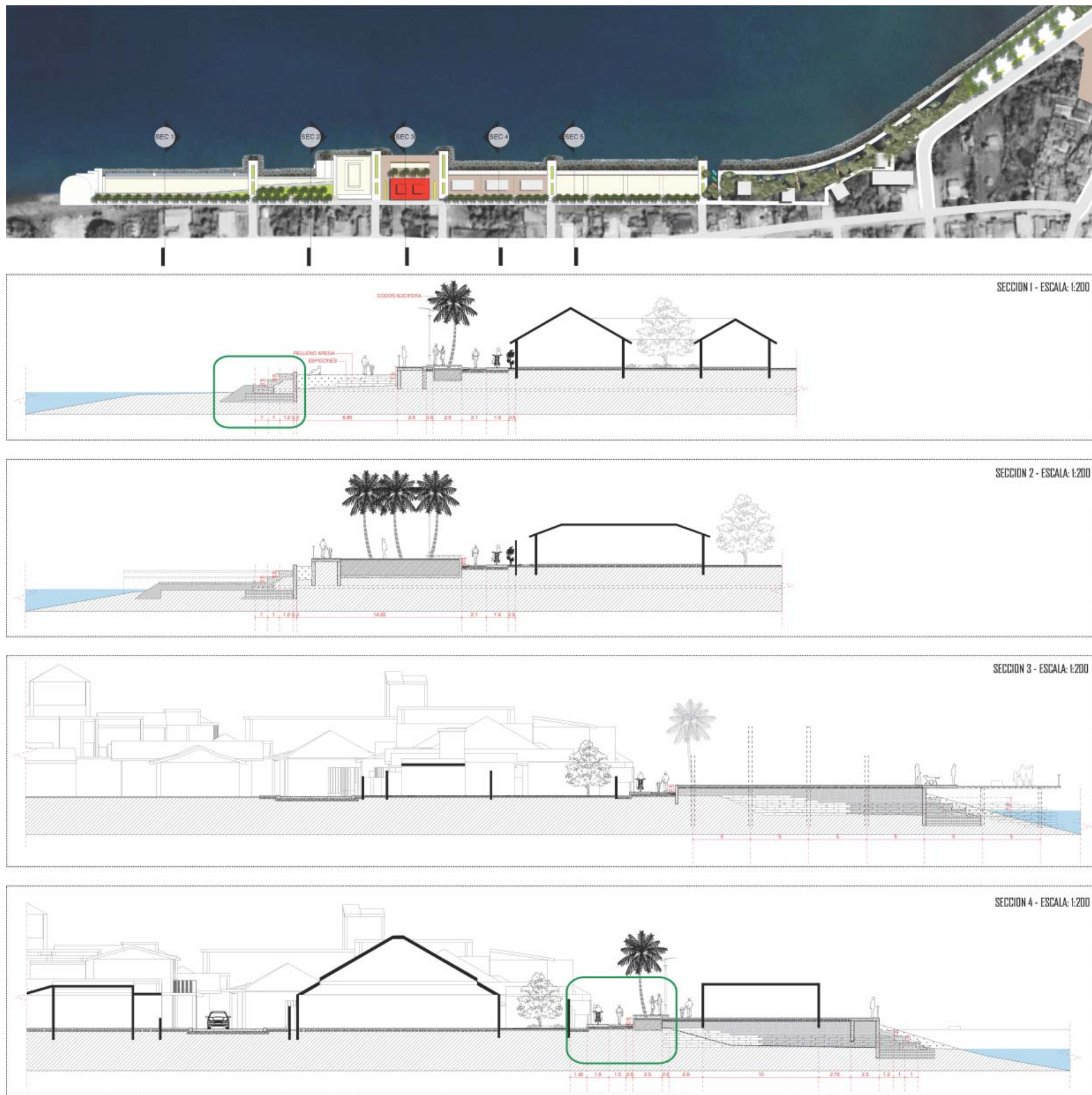
Figure 75: Sections. The sections show how the new development will be placed on top of the existing structures, thus creating a safe environment with a diversity of uses along the entire stretch of the walkway. Intellectual property of Re:Cua, Santo Domingo. Republished and translated with permission by Marcos Barinas. Original design panels are enclosed in their entirety in the Appendices chapter, pages 79-80.
