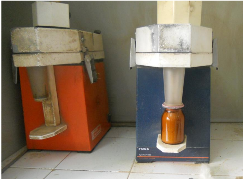
Figure 6. Grinder where all the samples were chopped into meal. Photo: Sofie Winding
