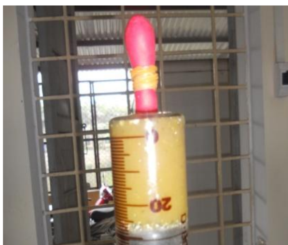
Figure 9. Glass syringe prepared with foliage mix, nitrate and rumen fluid. Photo: Sofie Winding
