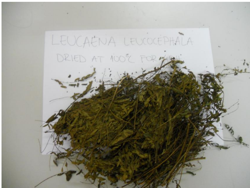
Figure 4. Foliage sample after dried in oven at 100° C for three hours. Photo: Sofie Winding
