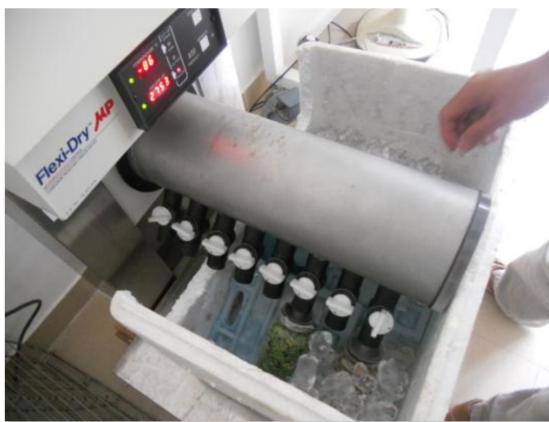
Figure 5. Freeze and vacuum machine in which samples from the foliage are placed in glass bottles. Underneath and around glass bottles ice is placed to help keep the samples cool. Photo: Sofie Winding
