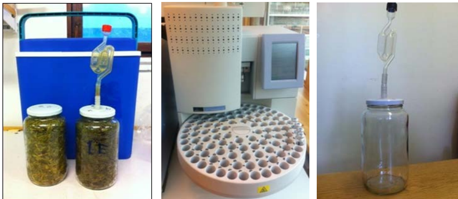
Picture 2. Silo lids with and without water lock (left); Perkin Elmer gas chromatograph (middle); CO 2 filled silos for experiment 2 (right).
