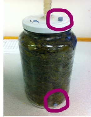
Picture 3 Silo lid sealed with two rubber stopper (pink marking)
