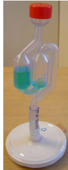
Picture 1. A water lock filled with water (blue) fitted on a metal lid of a glass jar.
