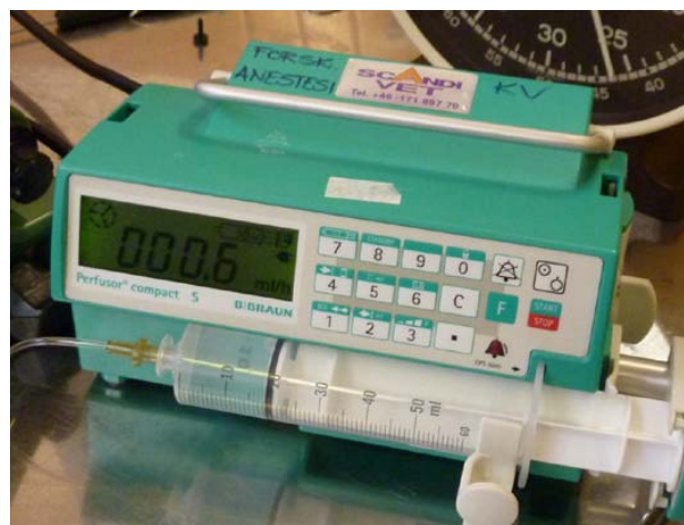
Fig. 2. TIVA infusion pump (Perfusor Compact B. Braun) with a 20 ml luer-lock syringe.
