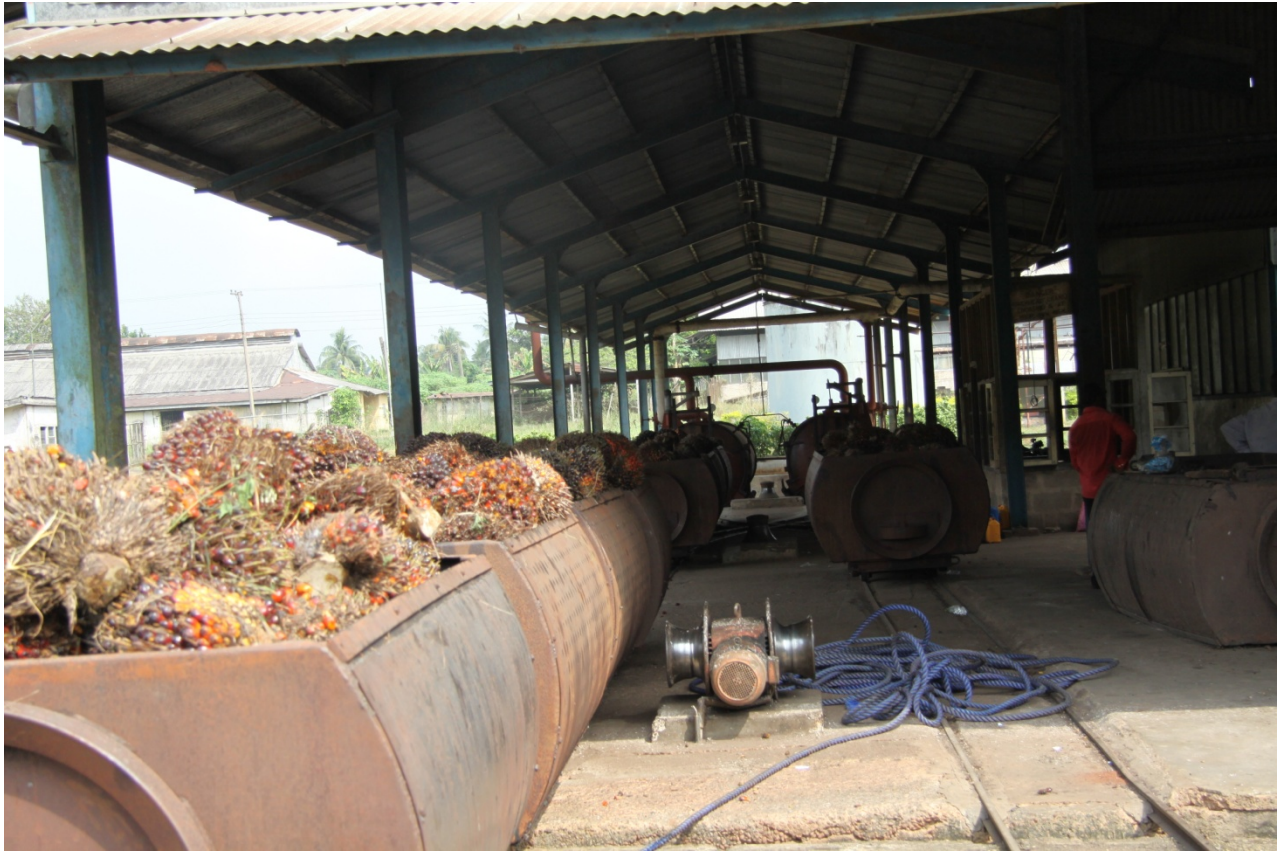
Conveyors of fruits bunch prior to fermentation at the section of automated milling press machine in Edo State
