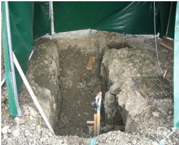
Figure 2. a) Initial pit. b) Side cavity and runoff collector.
