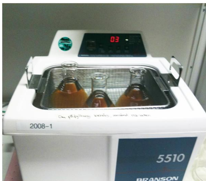
Figure 12. This picture indicates Sonication of Erlenmeyer flasks in present project. Sound waves were detached benthic diatoms from Erlenmeyer flasks. Sonication was carried out before each sample counting. Picture: S. Navid N.
