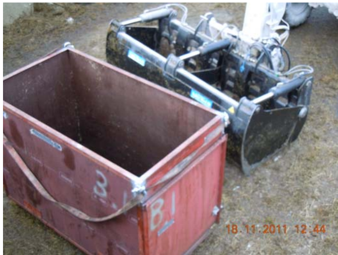
Figure 11. Block-cutter machine used at Ola, and the container used for weighing the blocks. Photo: Claes Jonsson
