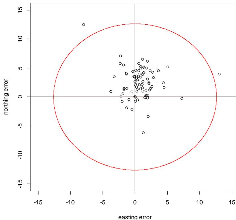
**Figure 12.** scatter plot of the easting (x) and northing (y) GPS errors (m) calculated by subtracting the differentially corrected GPS position from the real time GPS position measured in the field (Arbonaut dataset). The red circumference represents the Arbonaut's plot area in order to give an idea of the relevance of the GPS displacement across the dataset.
