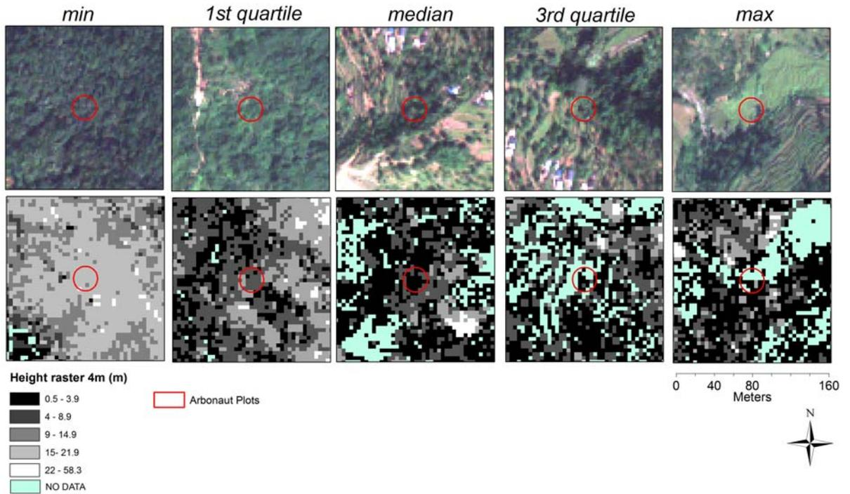
**Figure 4.** Range (minimum, 1<sup>st</sup> quartile, median, 3<sup>rd</sup> quartile, maximum values) of height Coefficient of Variation (CV) for the Arbonaut plots. No data values are pixels where there is no vegetation laser hit.
