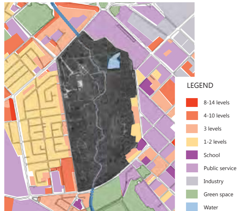
Figure 178: The plan shows building heights and land use of the area surrounding the park. Made by: Johanna Hagberg. Modified from: E-Urbanism, 2012.
