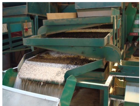
Picture 10. Beans are hulled to get green bean.
