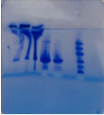
Figure 4. SDS-gradient gel analysis (8-25% acrylamide) after HiTrap Chelating HP chromatography. Stained with Coomassie Blue. Lane 1-7: Protein from peak-fractions. Lane 8: Low molecular weight marker. Size from the top: 97.0, 66.0, 45.0, 30.0, 20.1, and 14.4 kDa.
