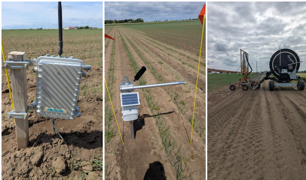
Figure 2.2. Field equipment used in the study. Left: the WM-17 telemetry unit connected to buried Watermark probes. Centre: CropX Evato. Right: the Rosenqvist hose reel and irrigation boom. The monitoring equipment was photographed on 8 June 2026 and the irrigation machinery on 17 June 2026; these are photograph dates, not installation dates.
