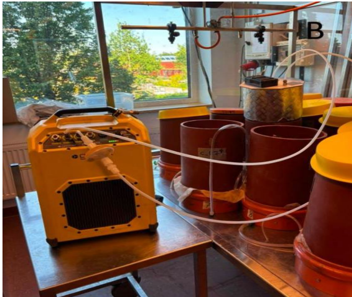
Figure 5: Gasmet GT5000 Terra Portable gas analyzer
