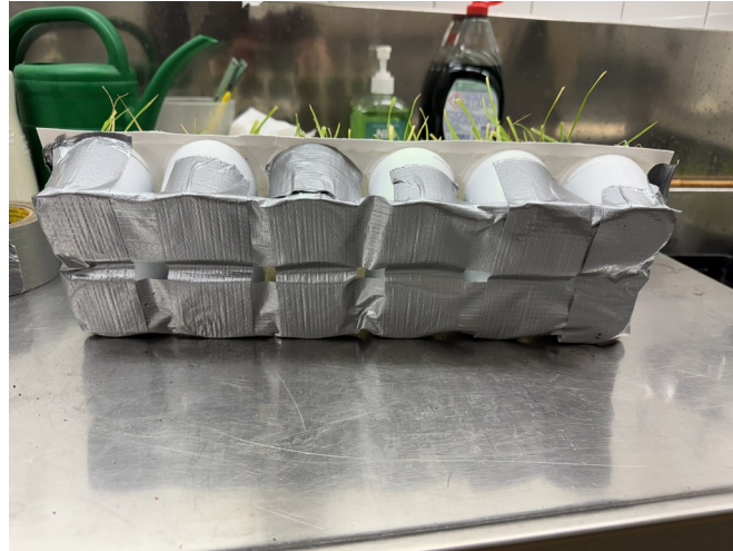
Figure 11. Tray holes sealed with two layers of duct tape to limit leakage during ice formation.
