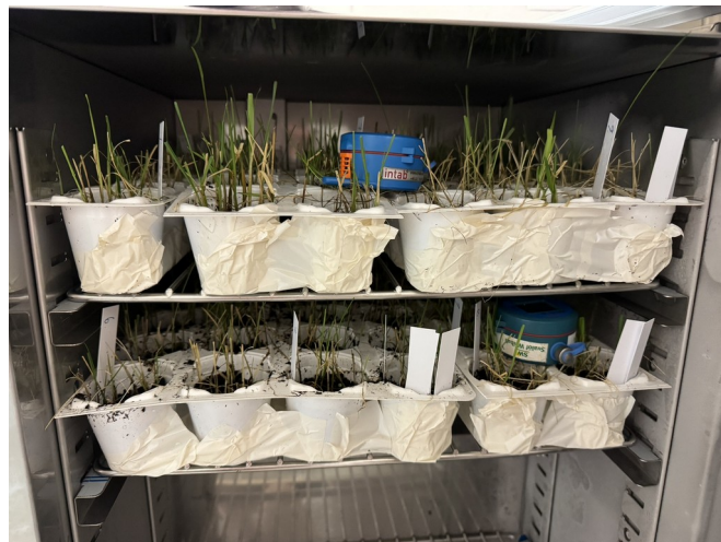
Figure 12. Placement of two temperature data loggers on the upper two sample shelves in one freezer; the same arrangement was used in both freezers.
