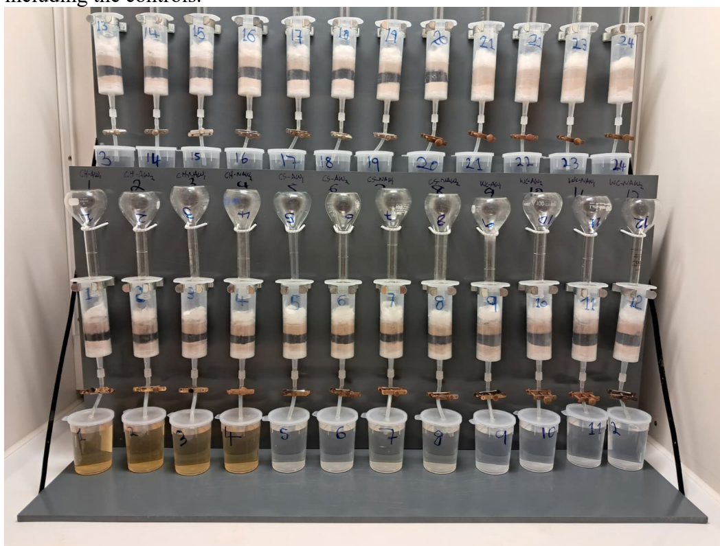
Figure 3. Experimental setup showing percolation columns filled with glass wool, sand and biochar–sand mixture and collecting beakers containing percolates.
