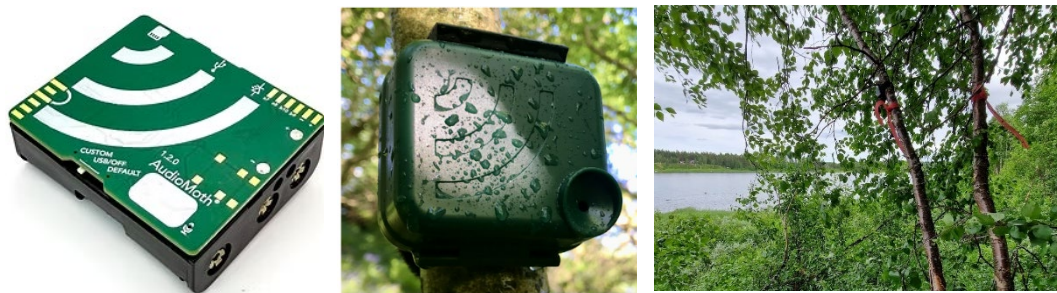
Figure 2. Left-to-right: AudioMoth device, mounted in waterproof case (©2025 Open Acoustic Devices) and deployed at site 30PaOR
