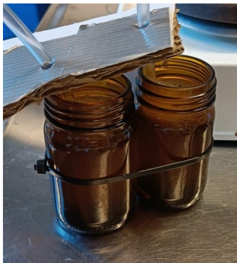
Figure 1. Picture of the experimental setup for Experiment 6 (Evaluation of Aeration Requirements) showing bottles U III and U IV with aeration tubes from an aquarium pump inserted through the bottle caps. Bottles U I and U II (not shown) were mixed using a magnetic stirrer without aeration and served as the stirred control condition.
