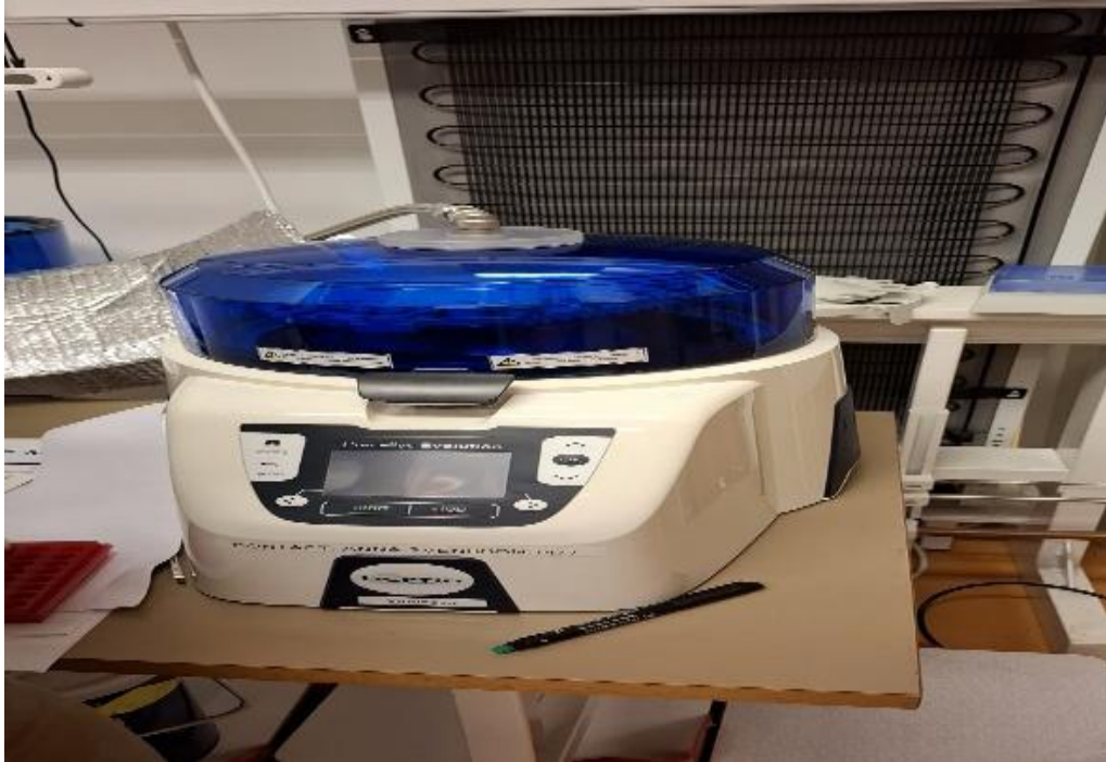
Figure 3. Precellys Evolution Touch homogenizer used for bead-beating lysis.
