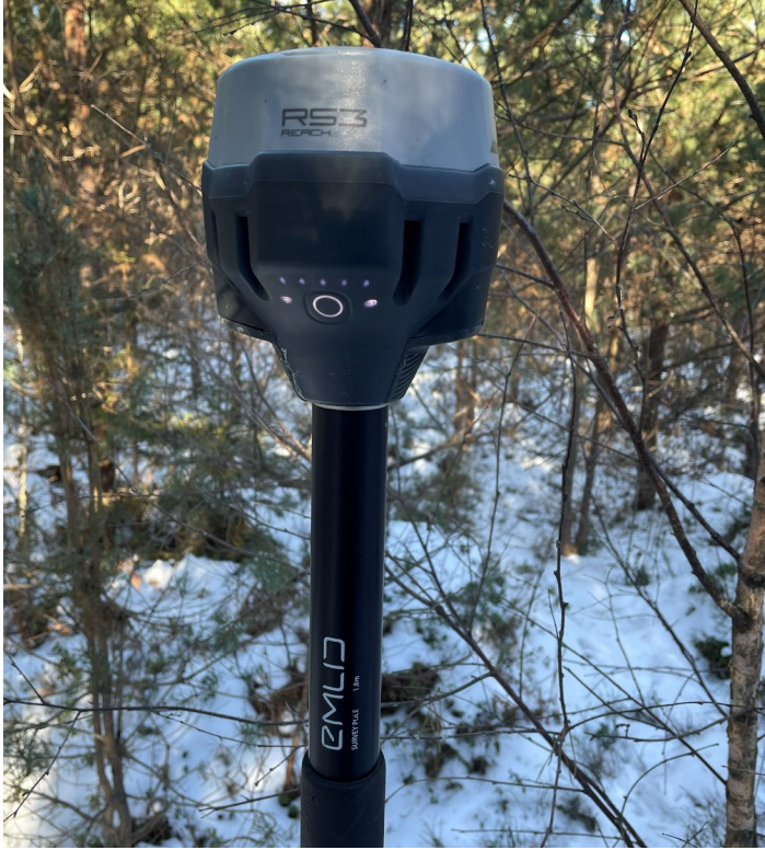
Figure 4. The Emlid Reach RS3 GNSS GPS- receiver in use during field work.
