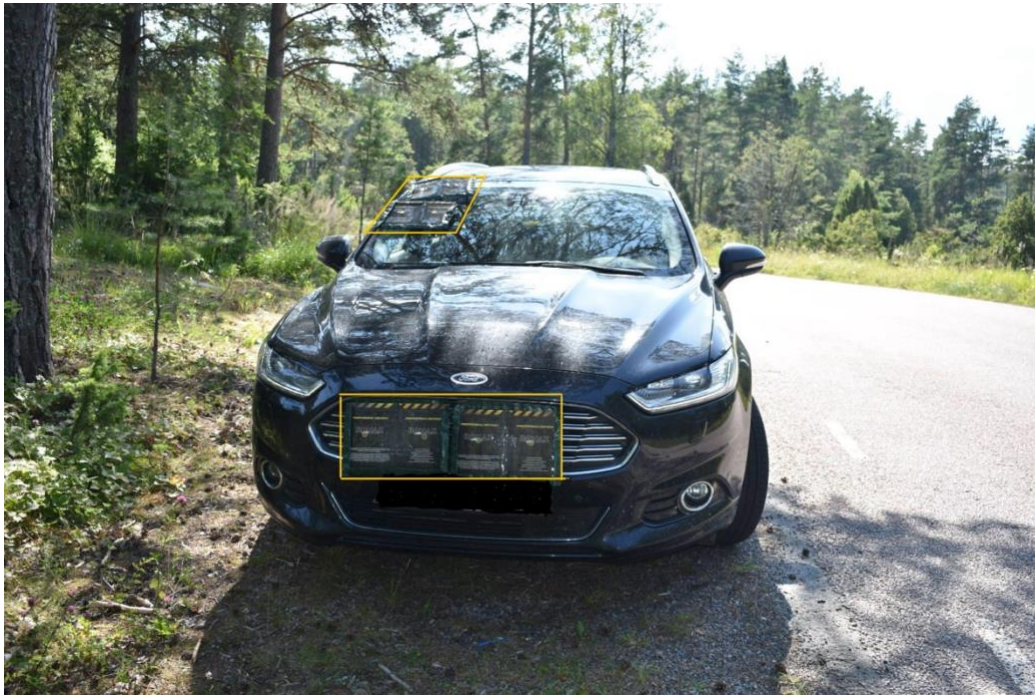
Figure 2: Sampling vehicle with four sticky traps – two on the front grill and two on the windshield (Photograph by Juliana Dániel-Ferreira).
