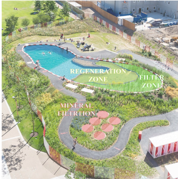
Figure 23. Aerial photo of King's Cross's layout and filtration systems (BD Landscape Architects, 2022); modified by author
