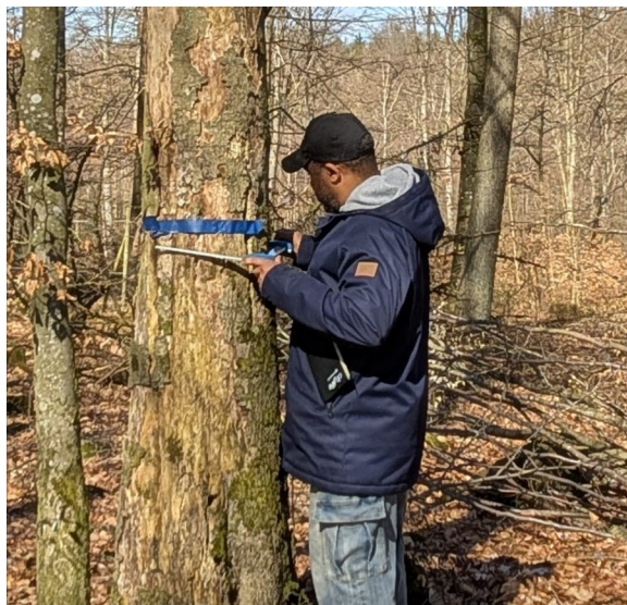
Figure 3. Measurement of the diameter at breast height (dbh) of standing deadwood using a calliper.
