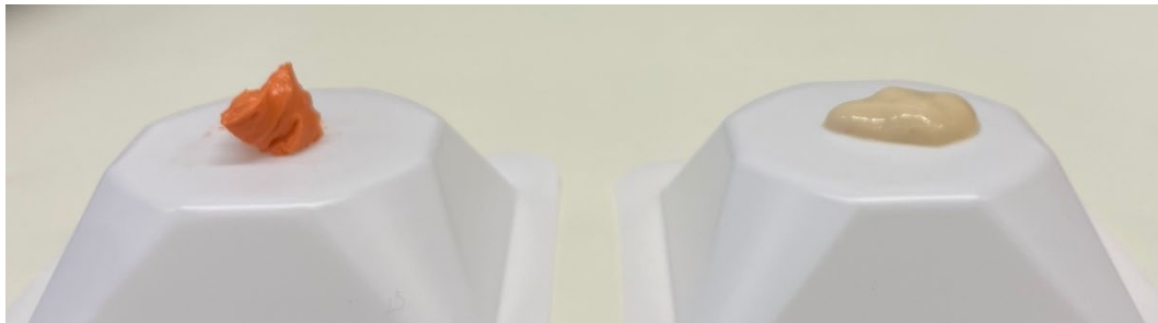
Figure 1. Protein gels after emulsification with yeast oil (left) and rapeseed oil (right), before heat induces gelation.
