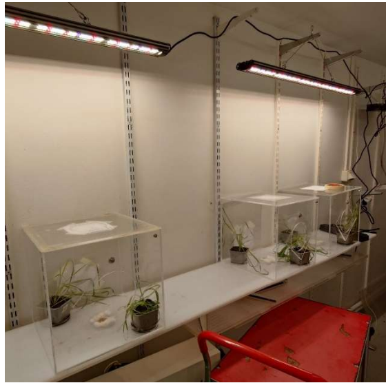
Figure 8. Climate chamber setup for E. corollae oviposition assay. Cages evenly placed under full spectrum LED for 24h.
