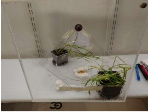
Figure 7. Cage setup for oviposition assay, E. corollae , oat and wheat infested with R. padi , feeding dish.
