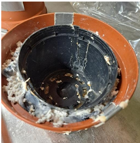
Figure 1. A mould was created by using two flowerpots of different size.
