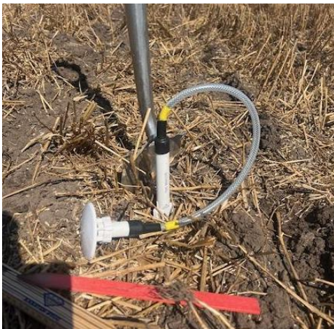
Figure 4: Data logger inserted in the soil
