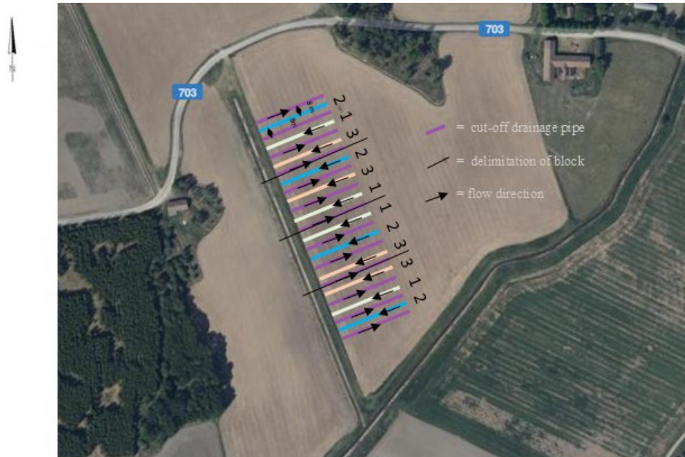
Figure 3. Map over the field trial where (1) is a perforated drainage pipe without envelope material, (2) is a perforated drainage pipe with a thick recycled fibre envelope and (3) is a perforated drainage pipe without envelope material with crushed rock (4-8 mm Ø) in the backfill. There are 16 metres between every drainage pipe. Between every drainage pipe is a cut-off drainage pipe.
