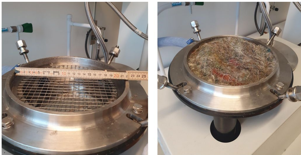
Figure 7. The diameter of the sieve of the machine to the left and the cut envelope in the sieve. Photo: Linnea Berggren Sjögård
