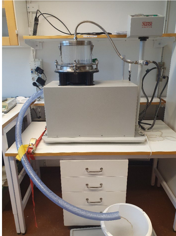
Figure 8. The machine TESTEX TG030 Geotextile opening size tester (wet sieving) is in process. Photo: Linnea Berggren Sjögård
