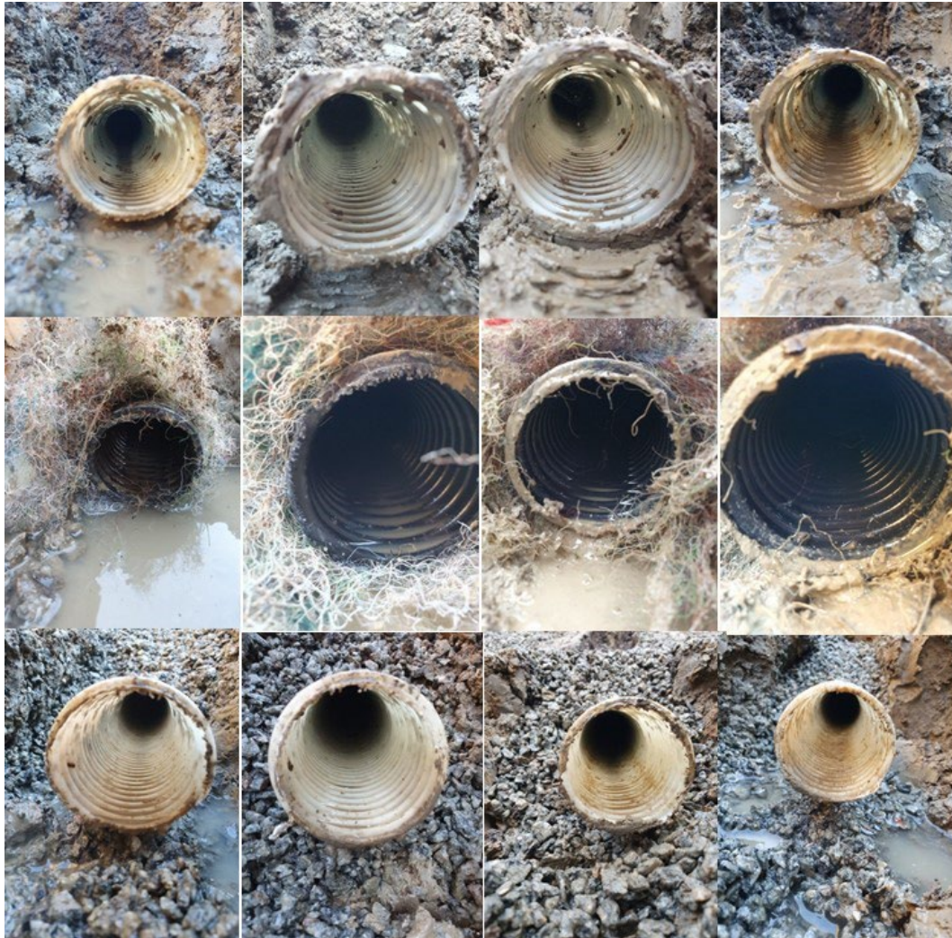
Figure 11. Picture of the inside of the drainage pipes from the excavation. Top: treatment 1 (no envelope) - plots 2, 6, 7 and 11. Middle: treatment 2 (synthetic envelope) - plots 1, 4, 8 and 12. Bottom: treatment 3 (crushed rock envelope) - plots 3, 5, 9 and 10. Photo: Linnea Berggren Sjögård
