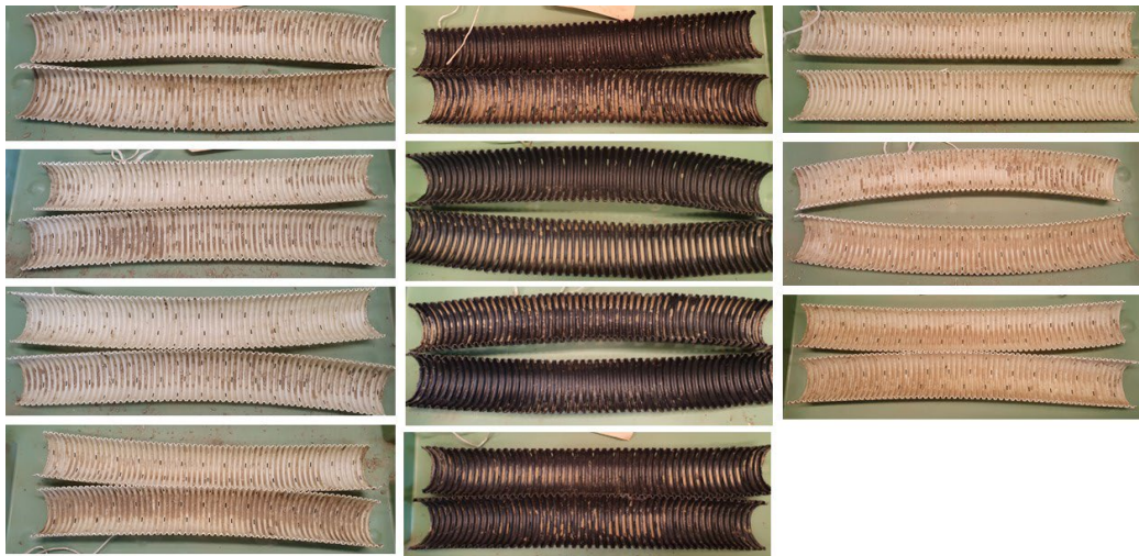
Figure 12. Demonstrates the amount of soil inside the pipes when they were cut open before cleaning. From left to right, treatments 1 (plots 2, 6, 7, 11), 2 (plots 1, 4, 8, 12) and 3 (plots 5, 9, 10). In treatment 3, the pipe from plot 3 was not photographed. Photo: Linnea Berggren Sjögård version
