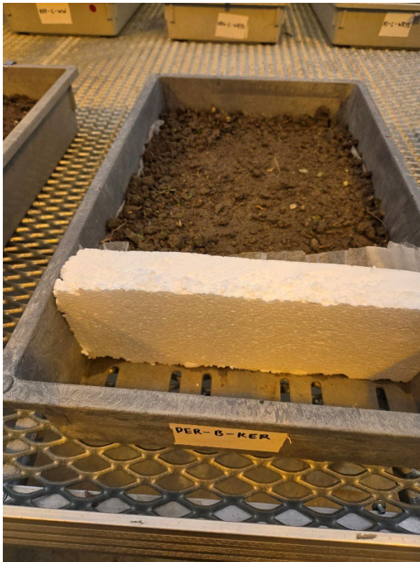
Figure 6: Soil tray setup with fiber cloth and Styrofoam block to adjust soil depth.
