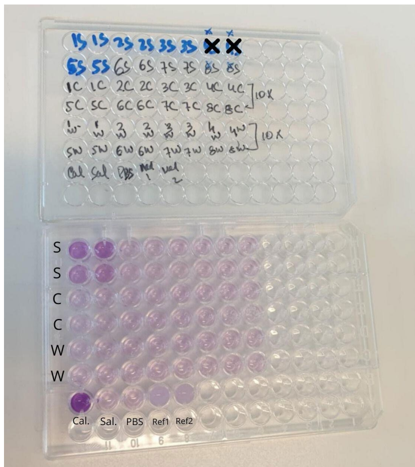
Figure 9. 5'NT test plate showing the samples and references to the sample placements. Sample 1-4 are milk based, where sample 1 contains all three bacterial strains, 2, 3 and 4 contains B. longum , L. lactis and L. reuteri respectively. Samples 5-8 are milk based with added AXOS where sample 5 contains all three bacterial strains and samples 6, 7 and 8 contains B. longum , L. lactis and L. reuteri respectively. These samples are analysed as supernatant (S), cells (C) and whole fermentate (W) in duplicates. Ref 1 and 2 is Milk and Milk+AXOS substrate respectively without bacterial strains added. Sal is 0.9% saline solution (blank calibrator) and Cal is calibrator. (Sample S4 (supernatant, B. longum ) are excluded because of pipetting error)
