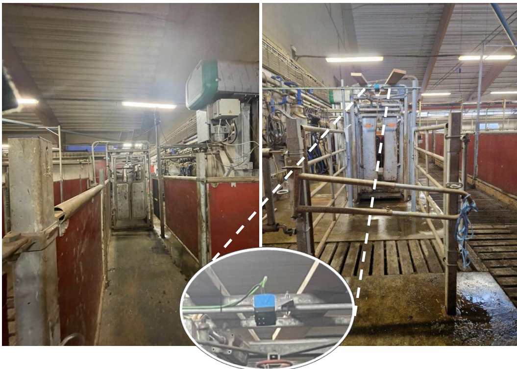
Figure 16 Entry (left) and exit (right) alleyway from the electronic weighing scale. Enlarged view of the TOF camera (middle).
