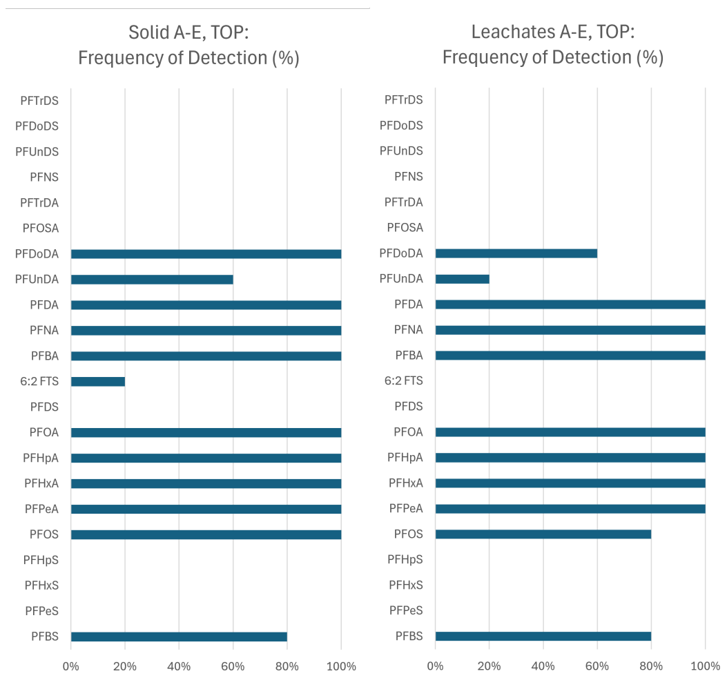
Figure 4. Detection frequency (%) of individual PFAS compounds across sampled SS (A-E), for solids (to the left) and leachates (to the right), analysed using TOP Assay (22 targets). A compound was considered detected in a given sludge if it was present above the laboratory reporting limits (RL) in at least one of three replicates analysed. The detection frequency reflects the number of sludge samples (A-E) in which each PFAS met this criterion.
