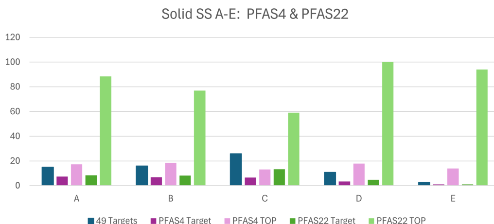
Figure 8. Calculated sums of PFAS 4 (pink) and PFAS 22 (green) from solid samples A-E, using target analysis (darker colour) and TOP Assay (lighter colour), in units ng/g. The total concentrations of target analysis, using 49 targets, above RL is also depicted in dark blue. REVAQ guidelines are set for 7.5 ng/g (PFAS 4) and 20 ng/g (PFAS 22), for comparison.
