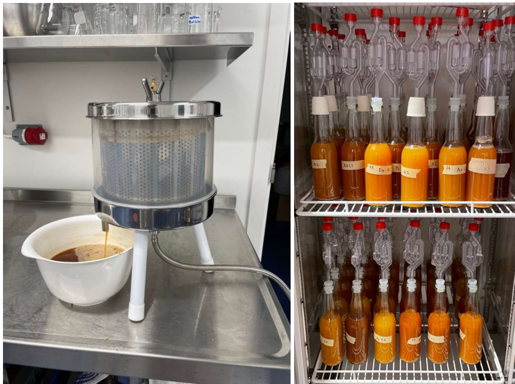
Figure 2: Processing and fermentation of the fruit. To the left: Pressing of the crushed fruit using a hydro press (Bladder Press frutty 6lt, Inderst GmbH, Italy). To the right: The bottles of juice, placed in a heating cabinet, to ferment at the start of the trial.
