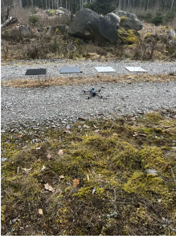
Figure 3. Ground control panels and DJI Mavic drone. Photo: Frida Linder.
